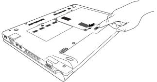
(Sample Illustration) Locking the battery release lock
